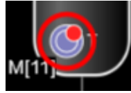
Fig. 6. An updated glyph in the geometric plant view. The small circle in the upper right corner shows the anomaly score of the known fault case time point, and the sensor is encircled in red to indicate the mismatch.
